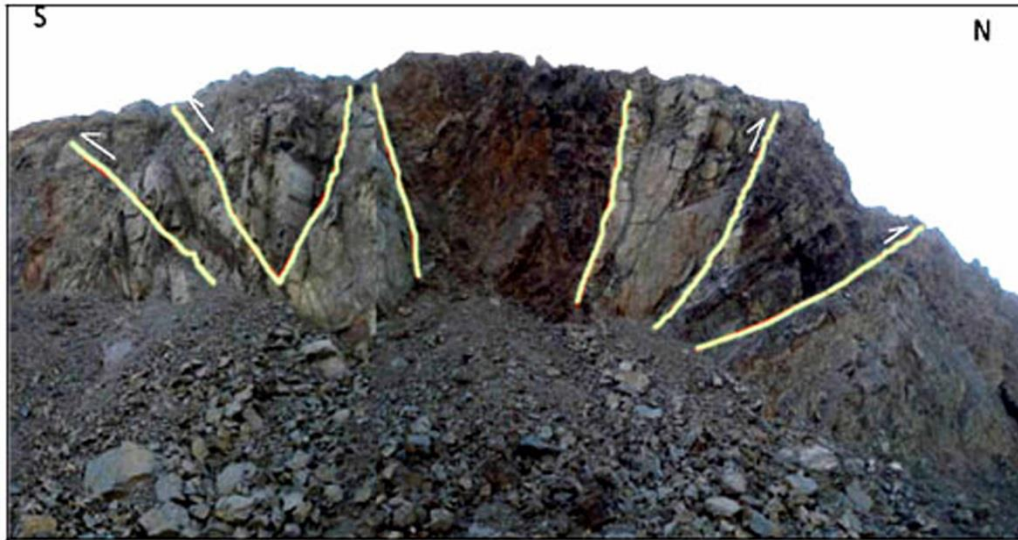
Fig. 2. Flower faults structure in the southwest wall of the Gol-Gohar mine (Hasanpoor et al., 2010).
